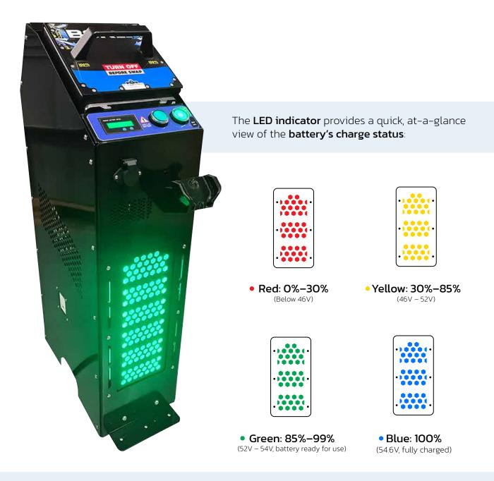
If the LED blinks, charging has stopped. Operators should check the RCCB, reset the dock by turning it off/on, and ensure that all fans are functioning.
